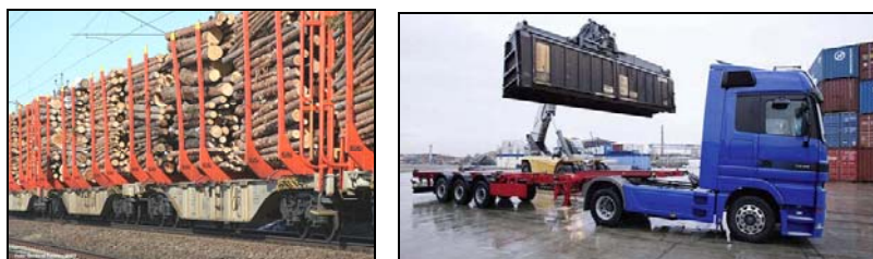
Fig.1 and 2: Standard container-wagons equipped with stanchions for timber transport in Sweden. (left; photo: G.Troche). Detachable superstructure of a freight wagon. The structure is not intended for transport on public roads and thus can utilize the full loading gauge of the railway. Standard intermodal handling equipment can be used in terminals (right).
