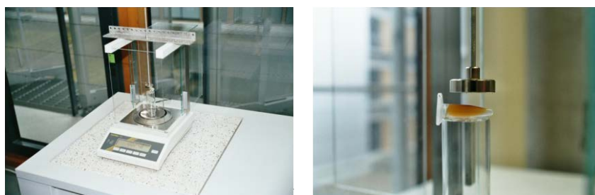
Figure 9. Measurement of the magnetic properties by a magnetic balance for SPIONs, magnetic MBs and magnetic capsules. left: whole setup; right: capsules during the attraction process.
