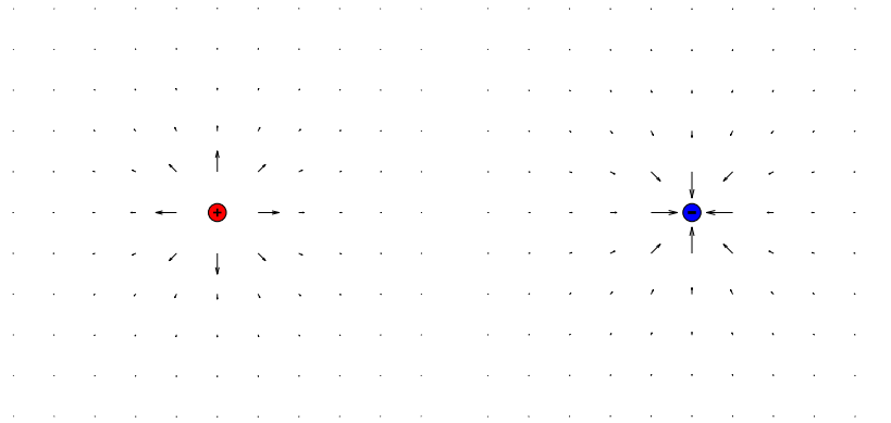
Figure 2.1: Electric field by a point charge. Left: positive charge. Right: negative charge.
