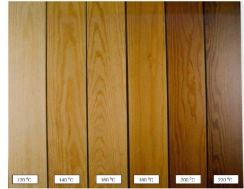
Figure 20-4. The colour of heat-treated pine. Treatment temperatures from 120 to 220°C at 20°C intervals. Treatment time (photo: VTT).
