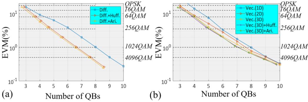
Figure 5. a) EVM versus number of QBs for differential coding and lossless coding; b) EVM versus number of QBs for vector coding and lossless coding.
