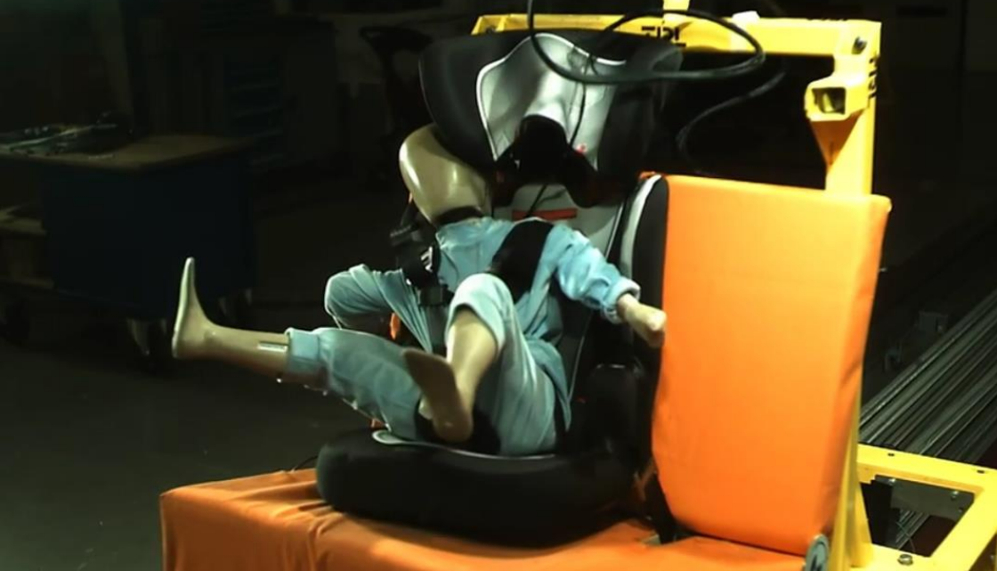
Source: ECE R44-04 test captured from video https://www.youtube.com/watch?v=cs18mg7Ux3c
