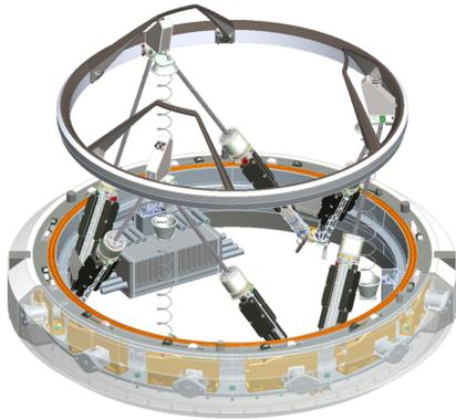
Fig. 2. ISS new docking ring [11]
