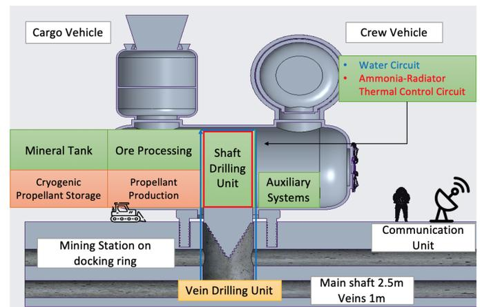
Fig. 1. System Architecture of the Mining Station
