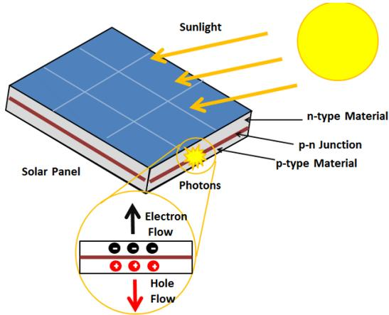
Fig. 4. Photovoltaic effect
