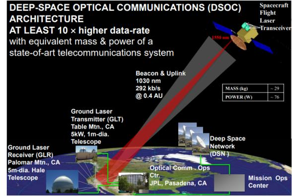
Fig. 3. Operational architecture for DSOC
