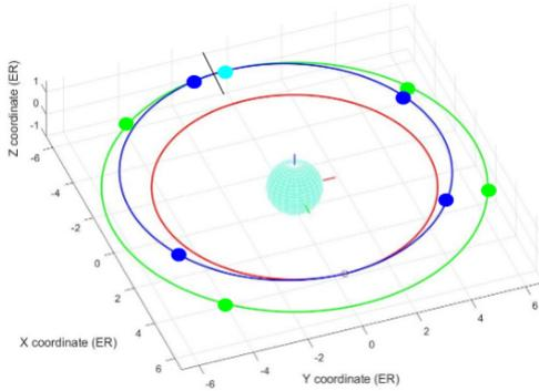
Figure 3: Hohmann Transfer between satellite 1 and satellite 2 both at GEO, but with an angle difference of  $9^\circ$ .
