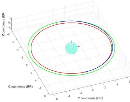
Figure 2: Hohmann Transfer between Chasing orbit (33 000 km) and GEO (35 851 km).
