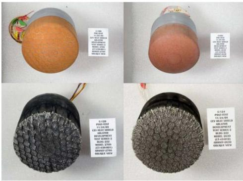
Fig. 9. Avcoat material pre- and post-ablation [5]
