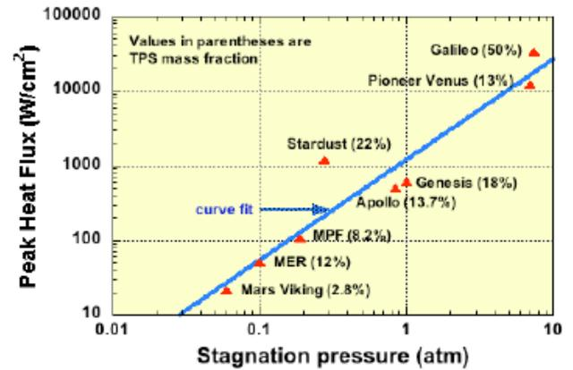
Figure 3: Mission environments for ablative TPS application
