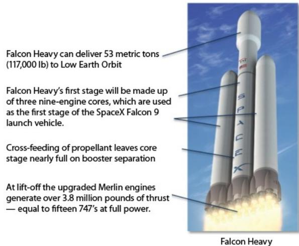
**Figure 1:** First stage of the Falcon 9 (top). The first stage of the Falcon heavy consists in three such stages. Artist view of the Falcon heavy in flight (bottom). Both images from [2]
