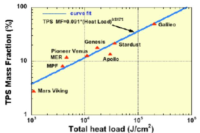
Figure 4: TPS mass fraction for prior ablative TPS missions
