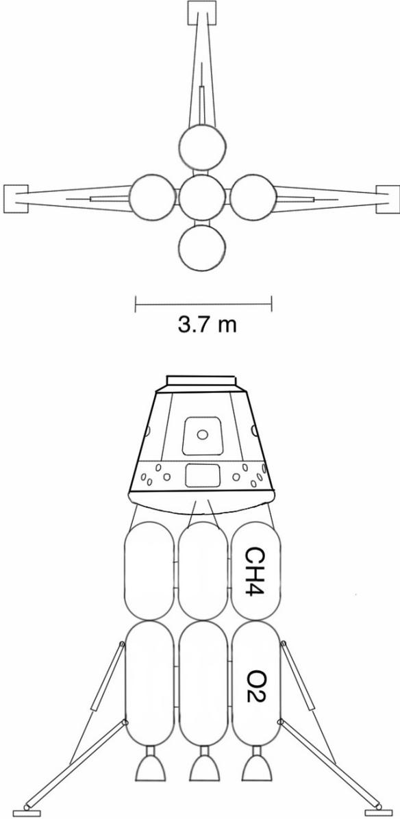
**Figure 5:** Dimensions of the lander based on the densities of liquid oxygen and liquid methane.
