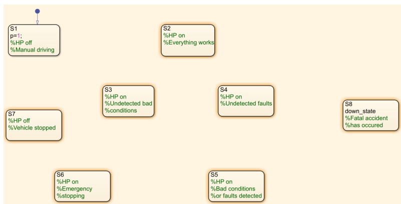
Figure 1: The states of the Highway pilot model
