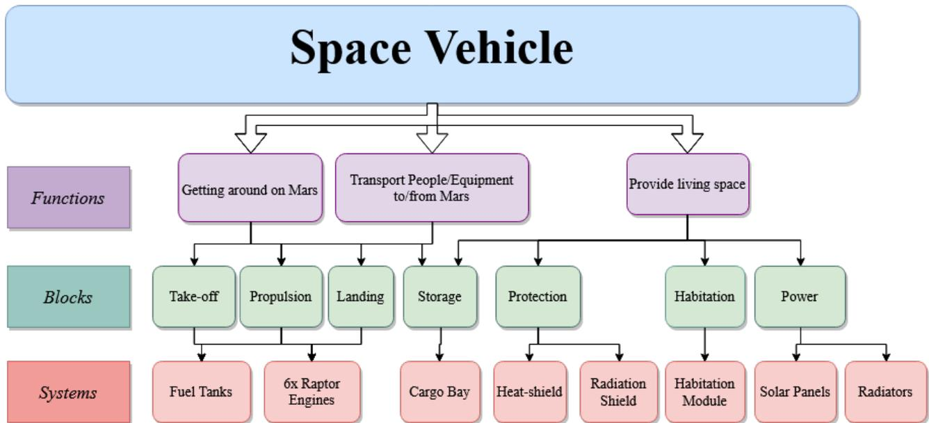
Figure 1: Functional diagram of the vehicle
