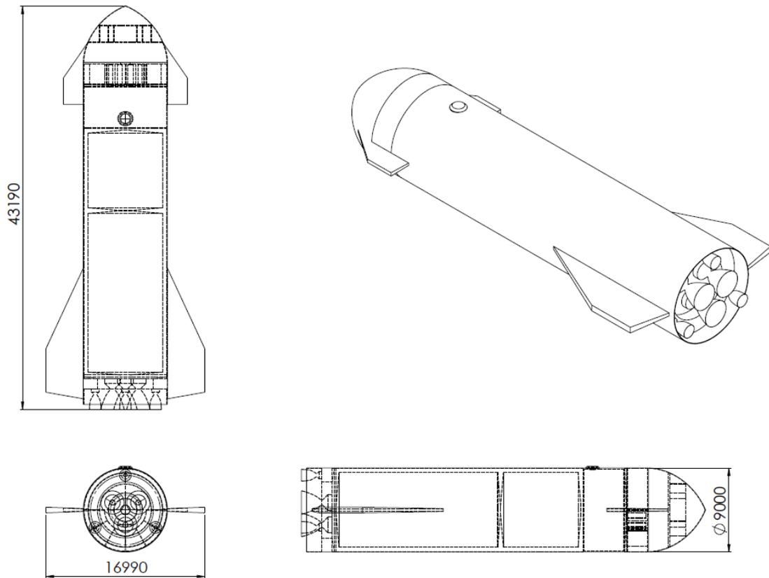
Figure 5: Engineering drawing of the space vehicle
