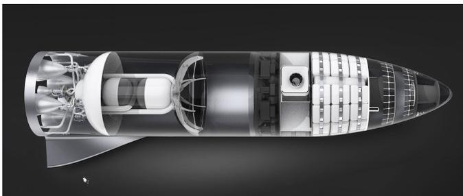
Figure 2: Starship spacecraft schematic of an old design iteration. Propulsion section and propellant tanks are on the left, crew and payload section on the right [6]
