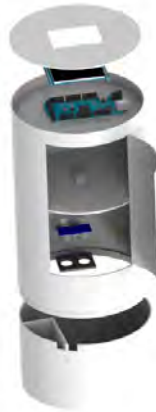
Figure 3.10: An exploded view of the prototype chassis along with some added components, created in Solid Edge [28].
