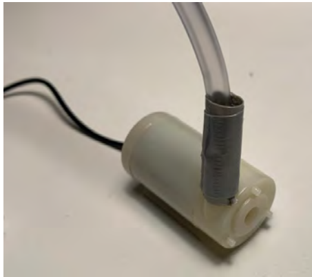
Figure 3.6: A 5V 1A water pump with 100 l/h flow rate, photo taken by Gustav Lindstrand.
