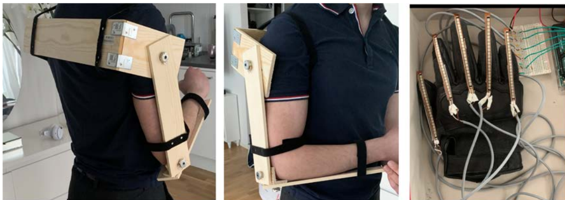
Figure 3.8: The control panel from two views and the glove with the flex sensors, pictures taken by the authors.
