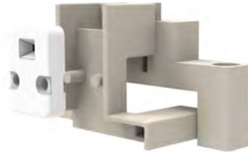
Figure 3.9: How the VL53L0X sensor from M5Stack could be mounted on the same elevator, designed in Solid Edge, image rendered in Keyshot
