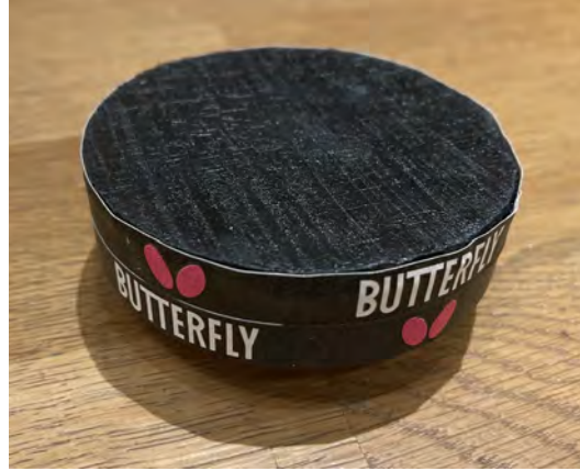
Figure 3.5: A close-up image of the spinning platform and the rubber added to increase friction. Picture taken by Axel Sacilotto
