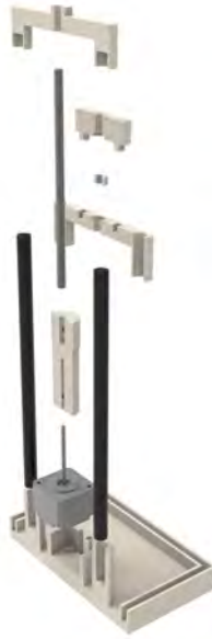
Figure 3.6: The elevator design, made in Solid Edge and image rendered in Keyshot
