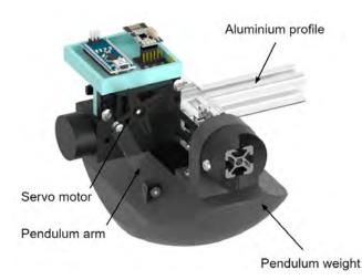
Figure 3.2. A CAD rendering of the pendulum. Created in Keyshot.
