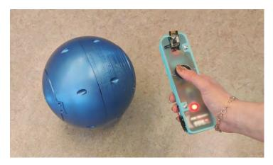
Figure 3.11. The final prototype, consisting of a dirigible bowling ball and the controlling remote. Picture taken by authors.
