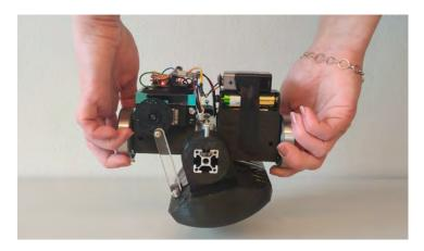
Figure 3.12. The inside mechanism showing the servo motor swinging the weighted pendulum. Picture taken by authors.
