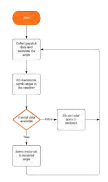
Figure 3.10. A flowchart for the Arduino code. Made with Lucidchart.
