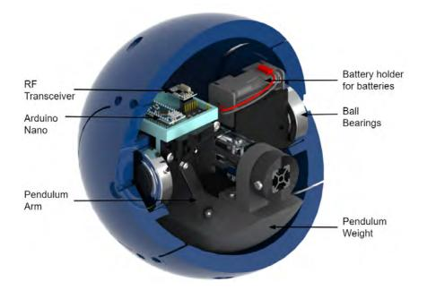
Figure 3.1. A CAD rendering of the robot. Created in Keyshot.
