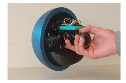
Figure 3.13. The mechanism inside the hollow bowling ball. Picture taken by authors.
