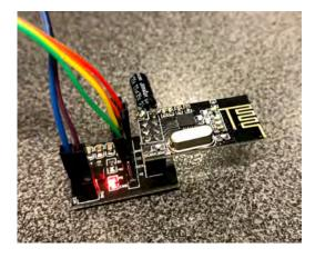
**Figure 3.8.** The nRF24L01+ module with a soldered on capacitor and an adapter module. Picture taken by authors.
