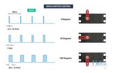
Figure 2.2. Correlation between the PWM and the shaft angle [9].
