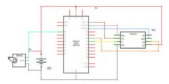
Figure E.1. The circuit diagram for the servo motor inside the sphere. Created in Fritzing.
