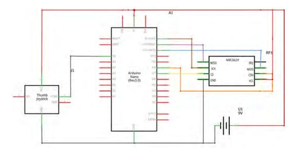
Figure E.2. The circuit diagram for the remote control. Created in Fritzing.
