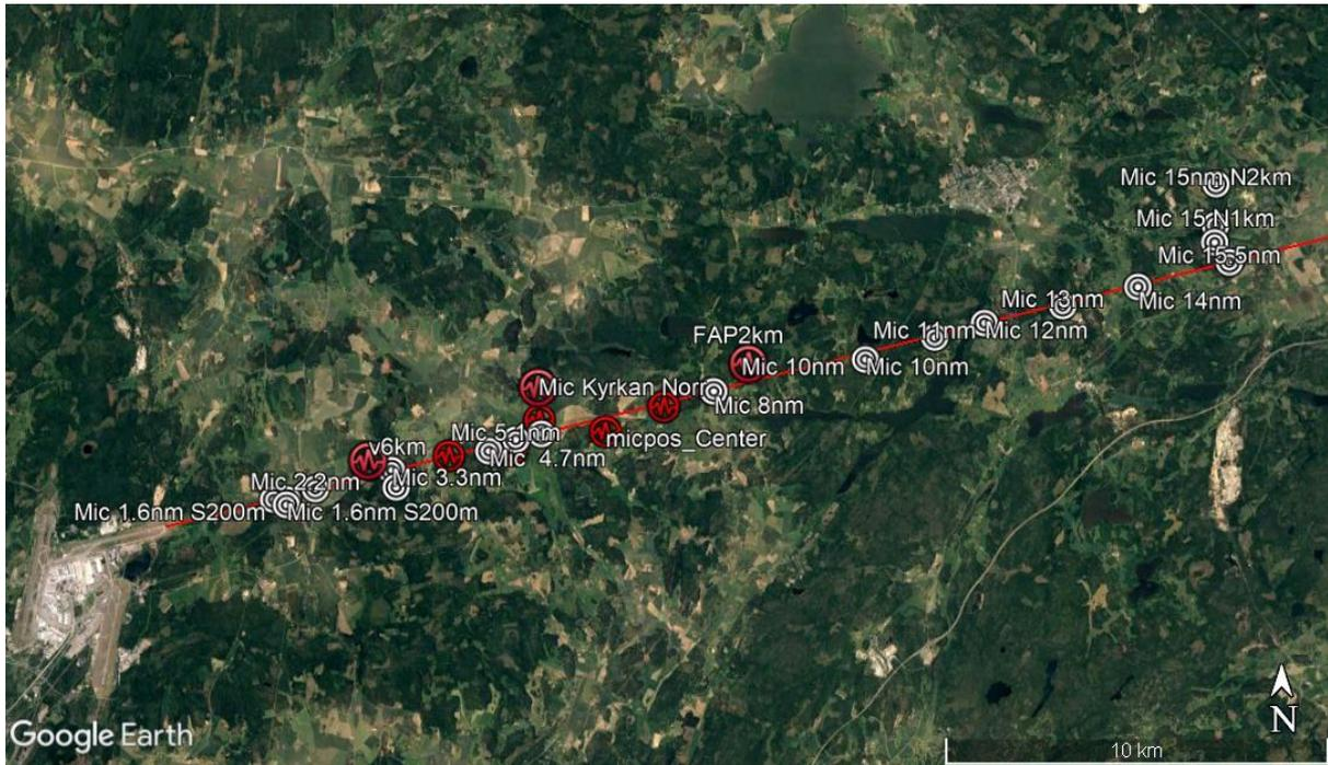
Figure 2: Satellite photograph over the measurement area. Arlanda can be seen at the bottom left corner. The red line, extending out 17 nm from runway 26, marks the ground track all aircraft followed when conducting the scheduled overflights. The red markers mark long term measurement positions for project ULLA and white markers mark the additional measurement positions for project ANT. The microphones are named after the position at which they are positioned.
