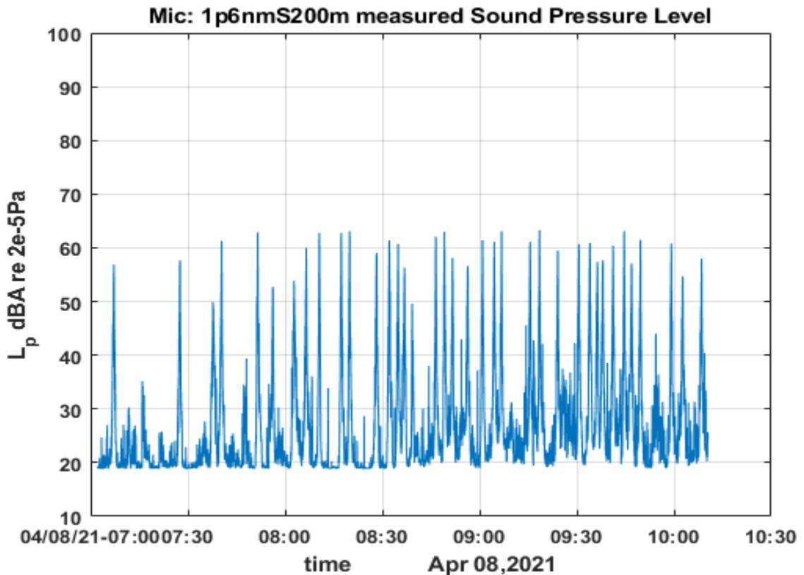
Figure: 4(b) Plot of sound pressure levels recorded by the microphone at 1.6 nautical miles away from the runway and 200m south of the trajectory. (a) is without weights while (b) is A-weighted.
