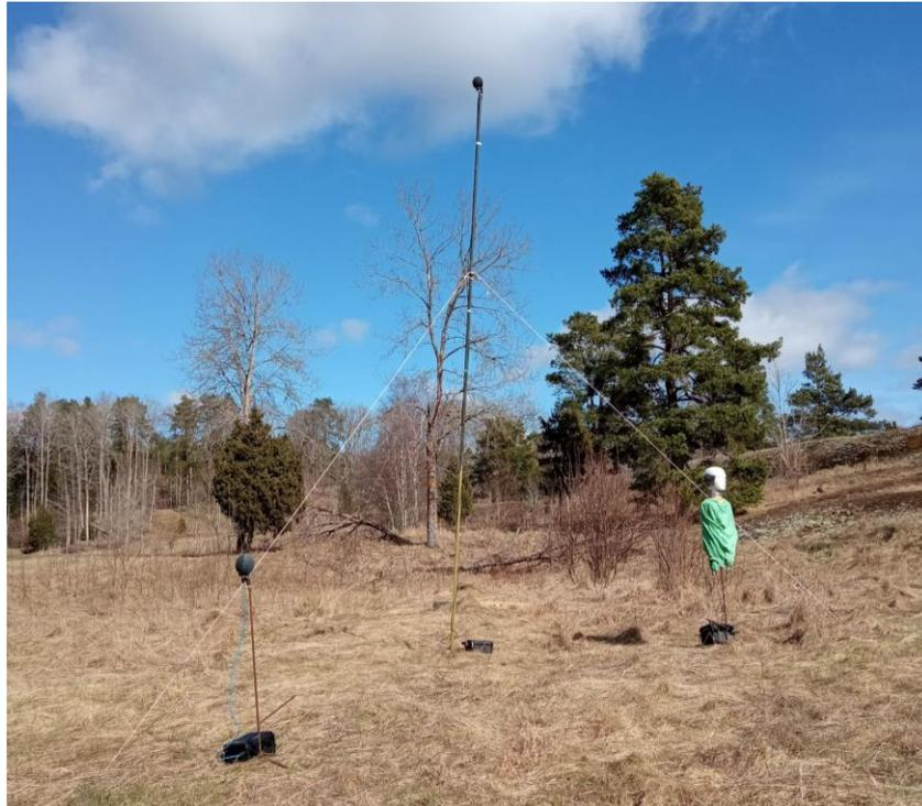
Figure 1: A photograph of the three different setups used during the measurements. The ordinary microphone setup can be seen at the bottom left side, the binaural recording setup can be seen to the right and in the middle the mast microphone is shown.
