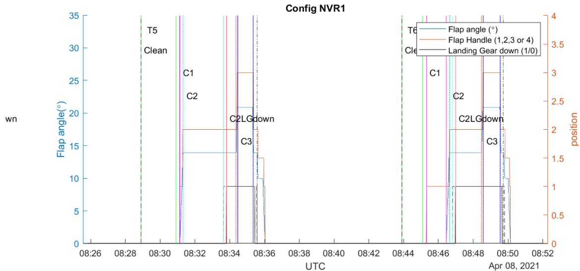
Figure 3: Excerpt from FDR-data showing a time record of configurational changes for two overflights. Clean, C1, C2, C2 and LGdown represents the different stages for high-lift devices and extension of landing gear.
