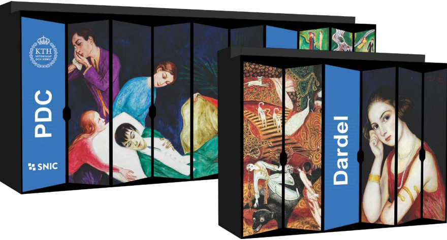
Above: To fit the extra cabinets in the PDC computer hall, a new row will be created in front of the row of cabinets for the first phase of Dardel. The new row for the second phase will consist of two compute cabinets on the left end and a narrower cooling distribution cabinet (which controls the water for cooling the system) on the right. In terms of the images on the door panels, two more paintings by Nils Dardel will be added and some of the panels will be rearranged, as shown above. The paintings that will be added are known as "Waterfall" and "Crime of Passion" and the full view of "Waterfall" can be seen on the cover page.
