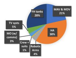
Fig. 3: Payload distribution without the propellant
