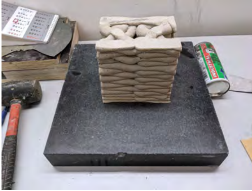
STEP 1: Flattening of top and base surfaces
