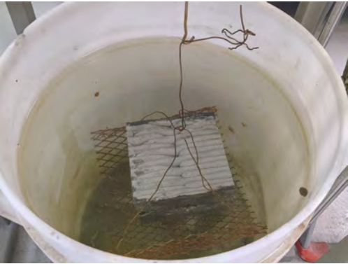
STEP 4: Measuring volume of specimen
