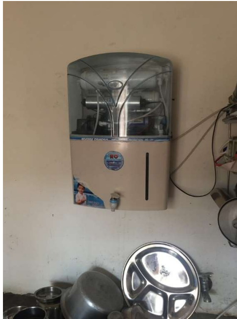
Figure 5: Reverse Osmosis Water Treatment Technology used at household level.
