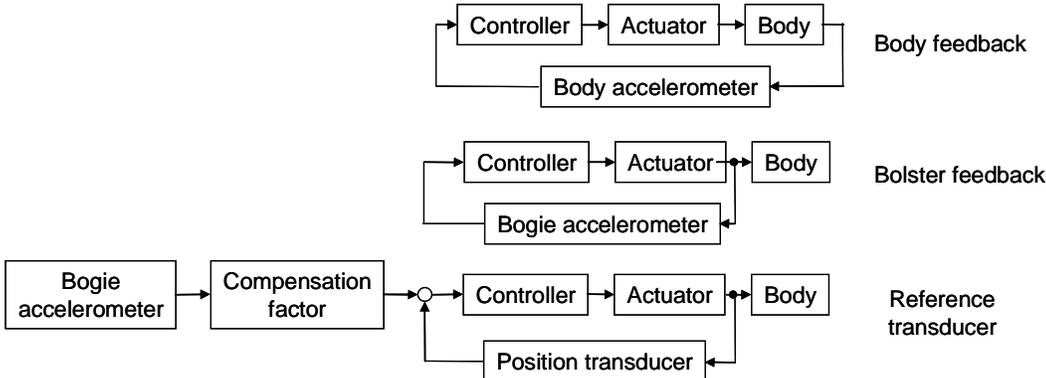
*Figure 7: Block diagram of tilting system layouts, Persson [13]*
