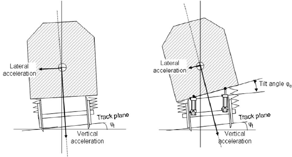
**Figure 2: The basic concept of tilting trains.** Despite the higher track plane acceleration for the tilting train (right), the lateral acceleration in the carbody is lower than for the non-tilting train (left), Persson [13].
