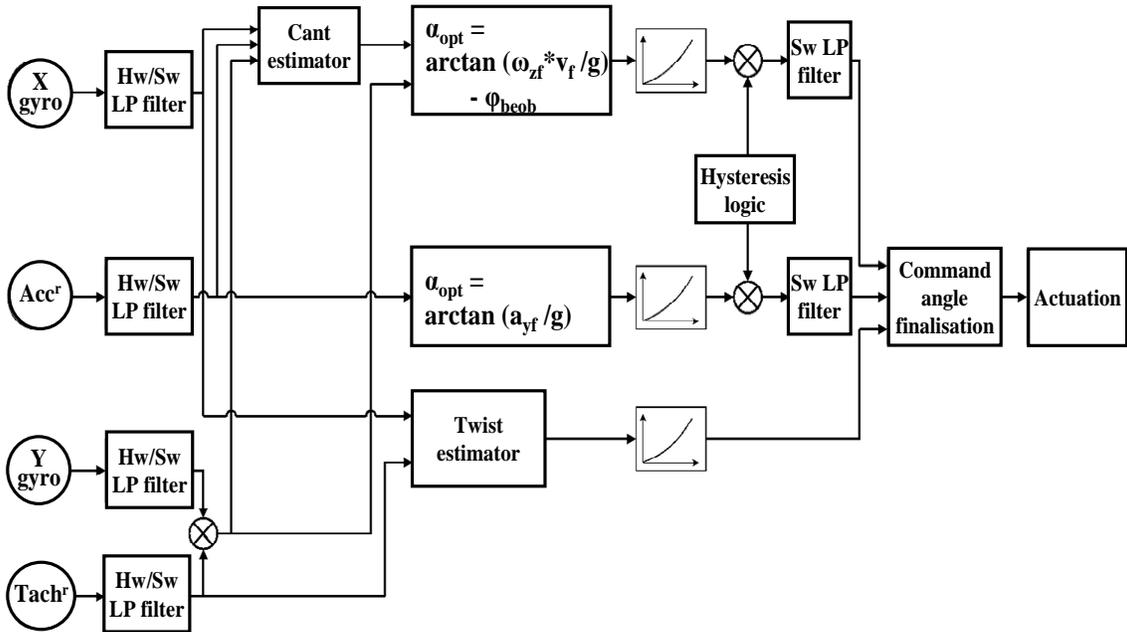
*Figure 8: Modern active tilting controller, Hauser [28].*
