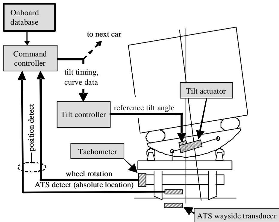
*Figure 9: Structure of controlled natural tilting, Sasaki [29].*
