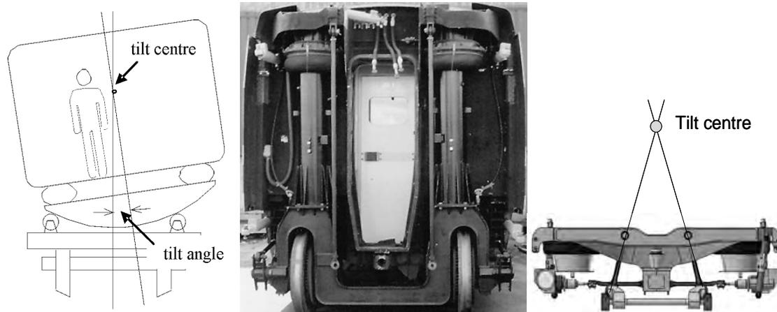
**Figure 4: Mechanical arrangements for natural tilt.** From left: swing bolster with circular guide, Persson et al. [4], high-positioned springs, Talgo [10] and inclined anti-roll bar links, Schneider [21].
