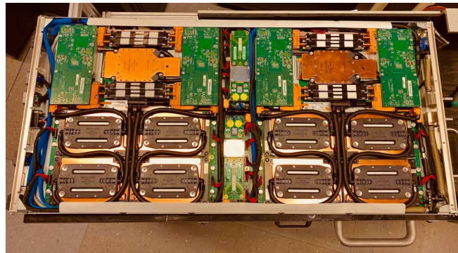
Above: PDC will receive three of these GPU blades as compensation, which will provide a total of six nodes with four GPUs each.
