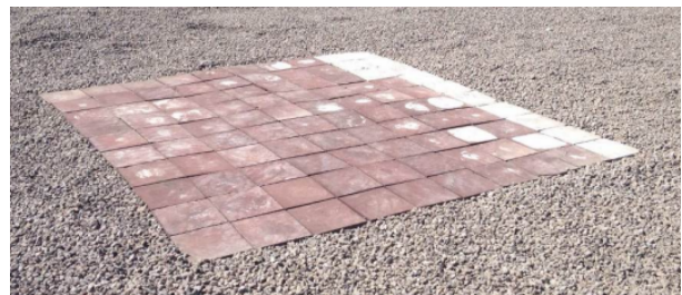
Figure 9: Experimental sample of a paved area realised by PICES rover
