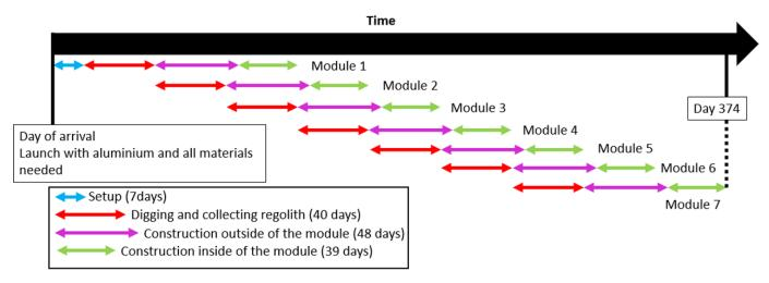
Fig. 9: Timeline of the construction of the base
