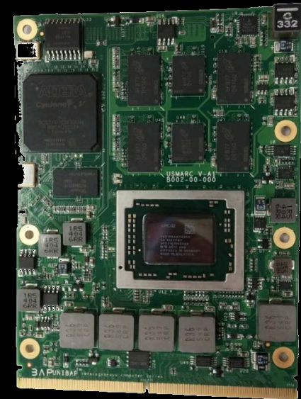
AMD R-series SOC “Merlin Falcon”, FP4 Altera Cyclone V GT Interconnect PCIe x4 v2.0 (20 GT/s) IOMMU, SVM, AVX2, HSA 1.0
