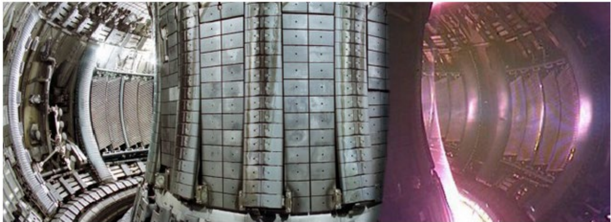
JET tokamak in Culham, England - with and without plasma that interacts with the wall.
