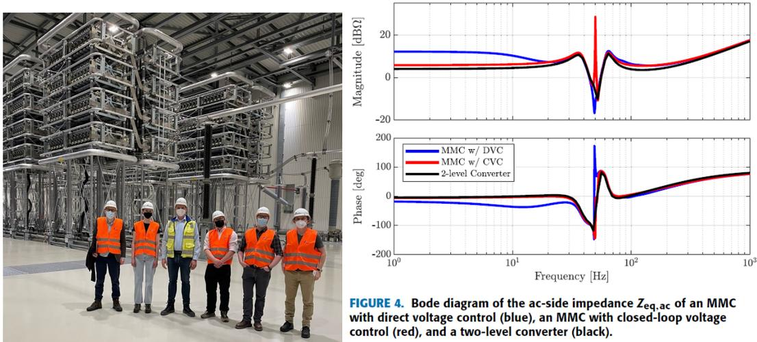
Picture of an HVDC converter (left) and equivalent impedance representation as Bode plot [3] (right)
