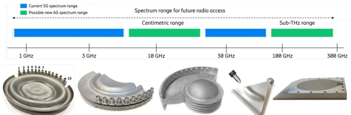
*Examples of FulMet metalenses produced by CNC milling and additive manufacturing techniques.*
