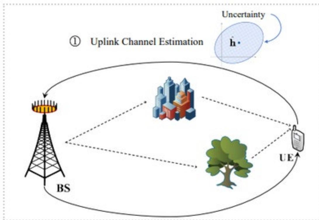
Channel estimation is a key step in wireless communication systems, but the estimates are affected by noise and uncertainty. To make reliable decisions, it is important not only to provide a point estimate of the channel but also to quantify the uncertainty of the estimate. Conformal Prediction (CP) is a general statistical method that can wrap around any estimator to provide prediction sets with guaranteed reliability.
