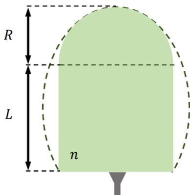
*Extended hemispherical lens schematic*
