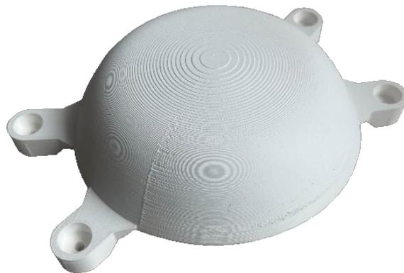
*Photo of a 3D printed dielectric lens*
