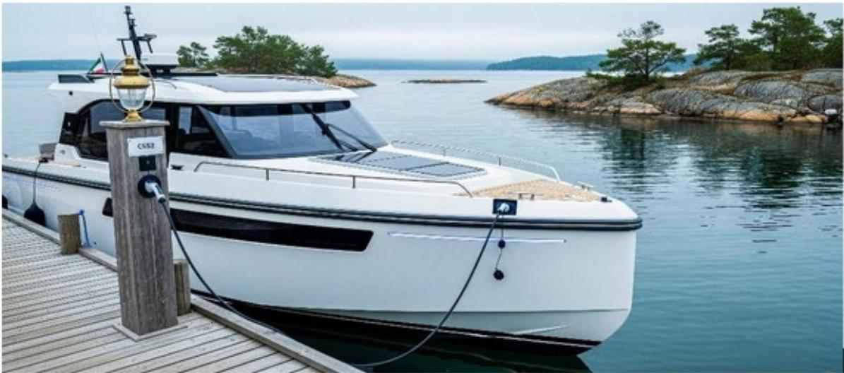
Given the high voltages and large currents found in EV charging systems it is essential that electrical safety aspects are rigorously investigated and handled from the marine perspective. Risk factors such as conductive salt water in contact with aluminium hulls create possible scenarios which are not encountered in terrestrial automotive applications.
