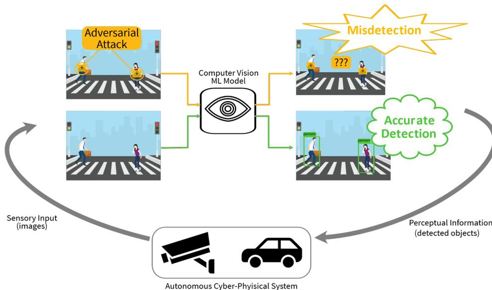
The performance and reliability of autonomous Cyber-Physical Systems (CPS) depend on (i) the accuracy of both the sensory information they acquire (e.g., camera) and (ii) the AI/ML algorithms they use to process it (e.g., object detection models). Adversarial attacks are sensory perturbations designed to mislead ML models, and thus pose a safety risk for autonomous CPS [1, 2, 3].
