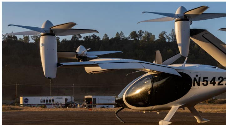
Figure 12. Picture of Joby air-taxi showing the tilting rotor system (K. Pascioni et al, 2022)
