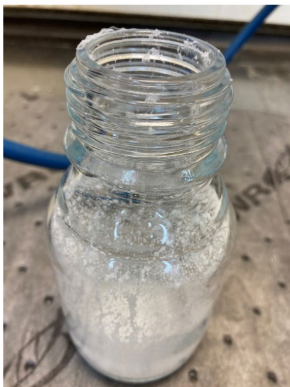
Figure 1. Glass jar containing polymerized HFO-1234yf (?). The foam was formed when a hose from a refrigerant cylinder with R513A was directed into the jar and the cylinder was briefly opened from the liquid side.
