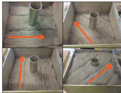
Figure 14: Metal wool and tube for HTF fluid[14].
