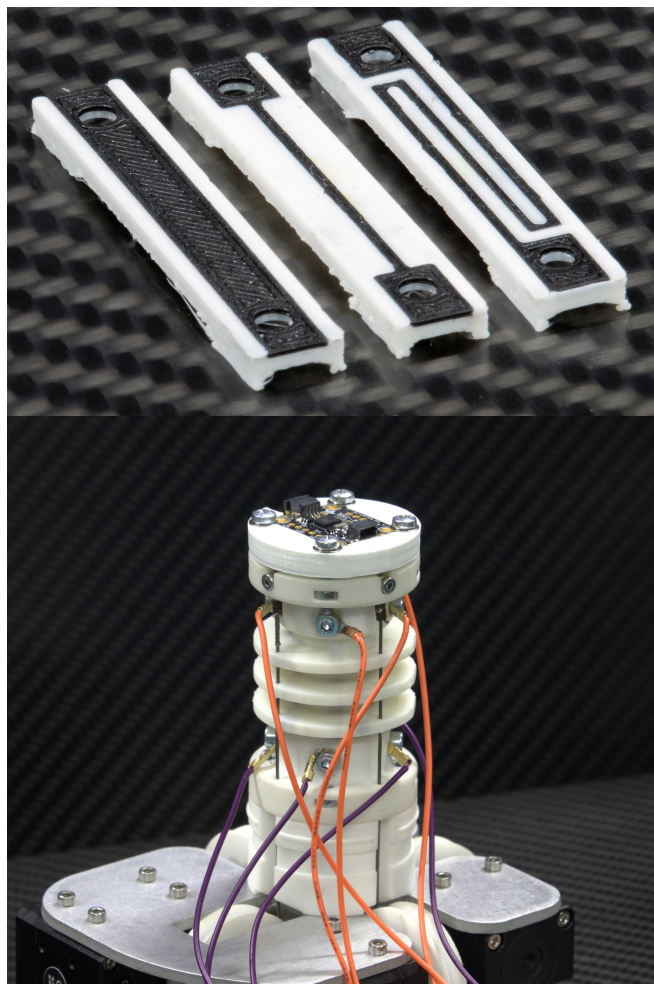
Fig. 4. (top) 3D-printed sensor prototypes fabricated with non-conductive (Shore 85A) and conductive (Shore 90A) TPU, corresponding to the geometries shown in Fig. 3. (bottom) Integrated smart SCA prototype without protective sleeve, with reference IMU mounted at the distal end. Visible wires correspond to temporary signal and ground connections used for evaluation.
