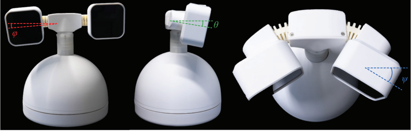
Fig. 2. Definition of the active rotation \psi and out-of-plane rotations \phi and \theta of the eyes in the revised HARU prototype. For clarity and comparison purposes, the deformation under load is shown on one eye to better illustrate the challenge addressed through the soft joint optimization presented in this work.
