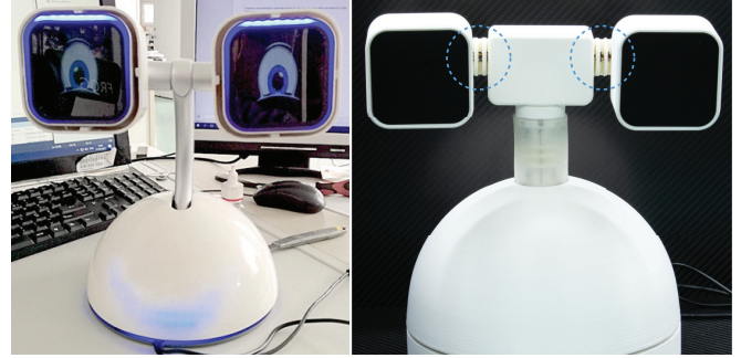
Fig. 1. (left) HARU as first presented in [3] and (right) the revised prototype structure incorporating soft joints in the head and eye structures, for enabling life-like motions and enhancing safety during interactions. This work is focused on the development and modeling of a soft continuum actuator for enabling the yaw motion of the eye structures (highlighted in blue and conceptually presented in Fig. 2).
