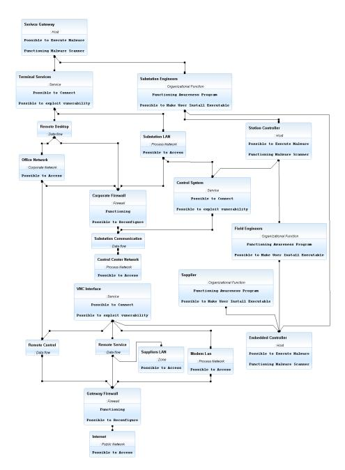
Fig. 7. Instantiated PRM for cyber security analysis. For readability only the classes and reference slots are shown in the picture, attribute relationships are hidden.
