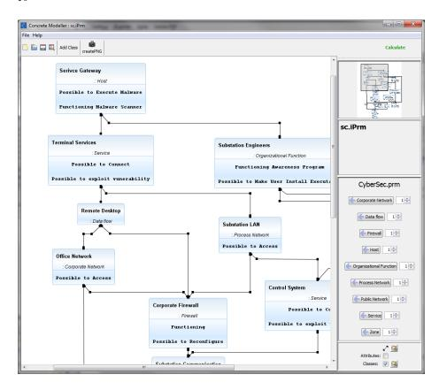
Fig. 6. Screen shot illustrating part of the instantiated PRM for cyber security analysis. For readability only the classes and reference slots are shown in the picture, attribute relationships are hidden.
