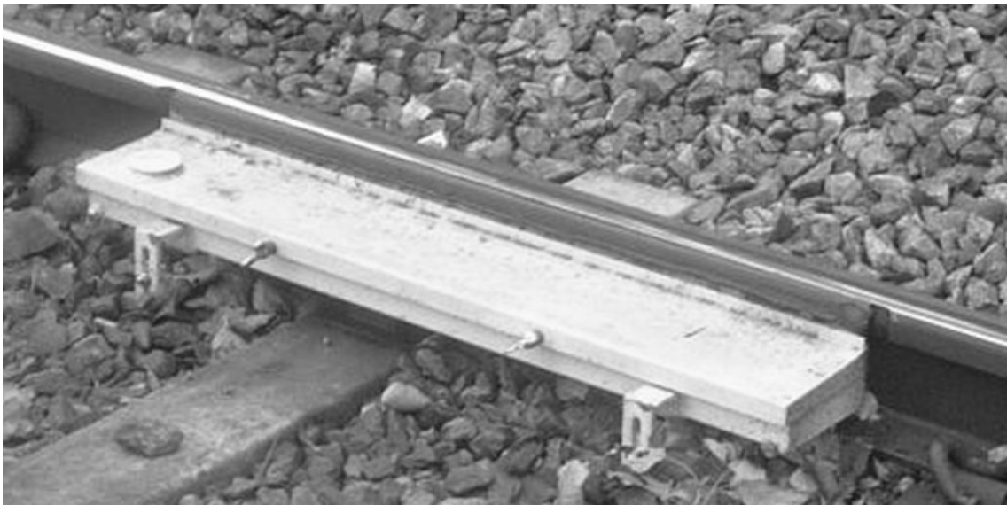
Figure 3-2 The lubricating device used at the embankment tracks of Tvärbanan. Photo by Faegh Adelpour.
