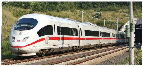
*Figure 8 The ICE3 train, designed for a maximum speed of 330 km/h Source: Wikipedia*
