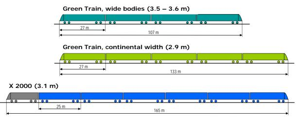
Figure 6 Green Train wide bodies convey more passengers per meter of length than an ordinary train.
