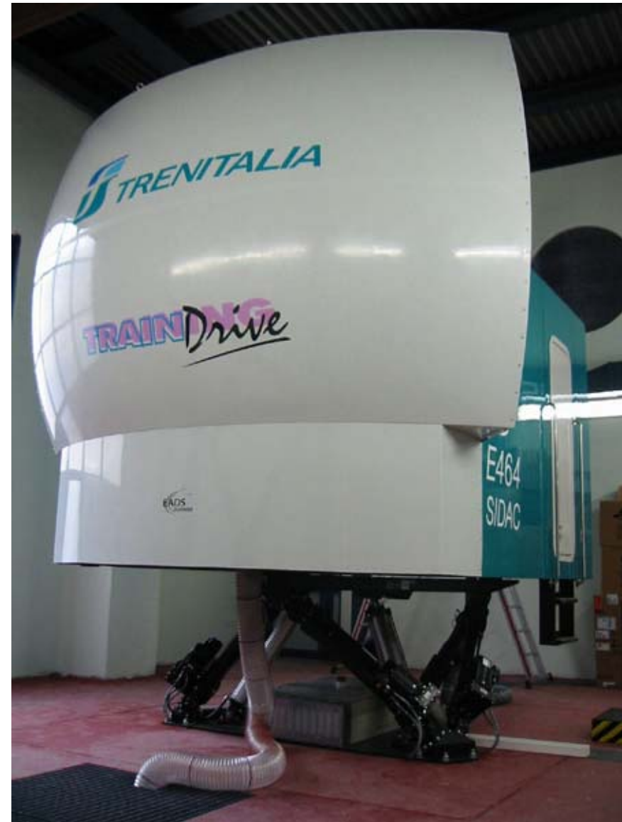
Full scale simulator: cabin and motion
