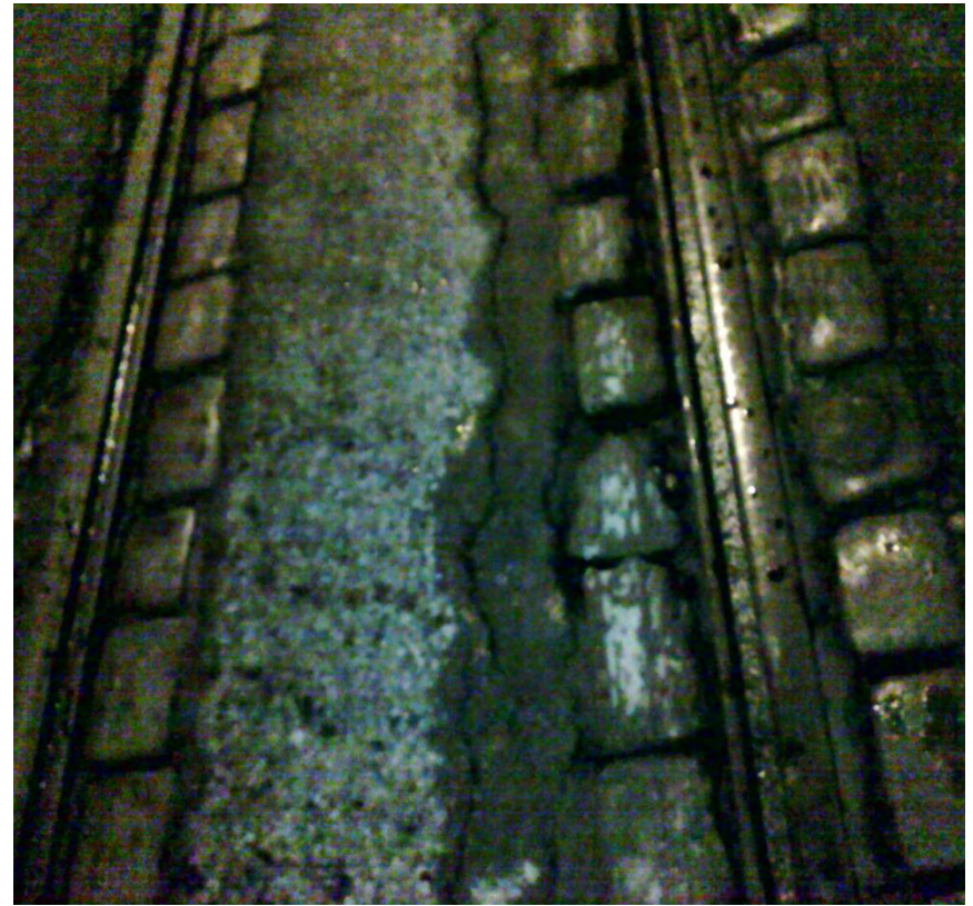
Droplets of \text{MgCl}_2 spread on the track ( 25 \text{ g/m}^2 )
