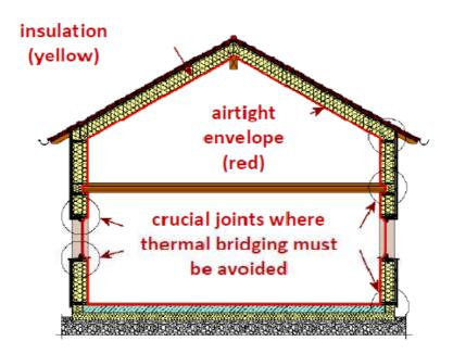
**Figure 3.** Passive house concept: airtight building envelope (original illustration: Passive House Institute, passipedia, <u>www.passipedia.org</u>; modified by author)
