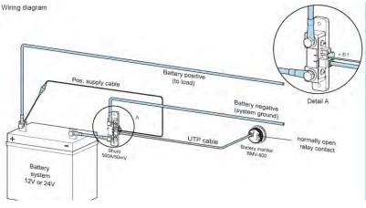
Figure 13 : Diagram for mounting the BMV
