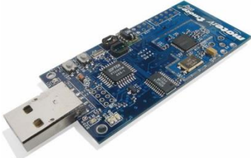
Fig. 7. Figure displaying a Tmote which is used for communication between the controller and the quadrotor.
