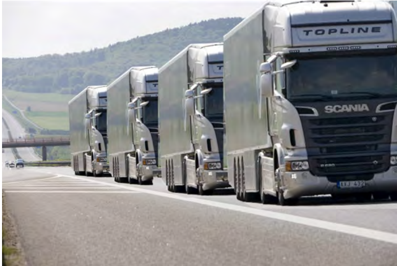
Figure 1.3: Usual formation of a platoon (courtesy of Scania).
