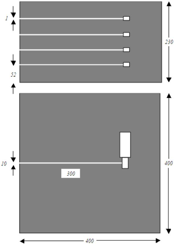
**Fig. 6:** An illustration of the collimator package, including four gamma-ray detectors, being used in the test platform. The width, height and length are 230 mm, 400 mm and 400 mm respectively. The collimator slits are 300 mm long. The slits are exchangeable so that the slit width and height can be selected. At the test measurements a width of 1 mm and a height of 10 mm were used.
