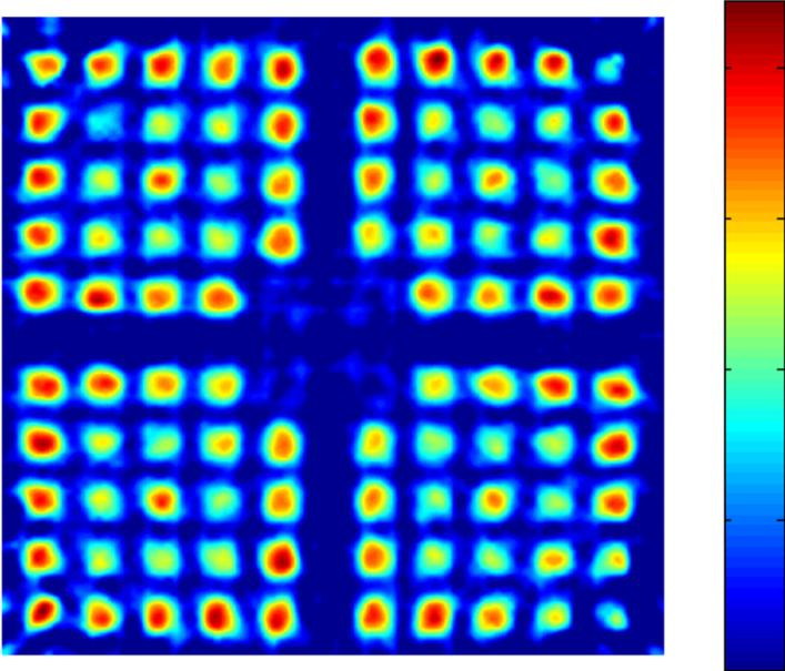
**Fig. 4:** Tomographic image obtained when analysing data from the measurement of a SVEA96-S fuel assembly at the Forsmark power plant in 2002 [8]. All 96 fuel rods are clearly distinguishable from the background.
