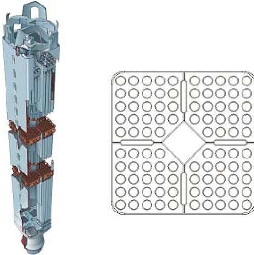
**Fig. 1:** Illustration of a BWR fuel assembly of the SVEA96-S type (left) and its cross section (right). This fuel type contains 96 fuel rods. The mass is about 200 kg, the length is about 4 m and the cross section is about  $15 \times 15 \text{ cm}^2$ .
