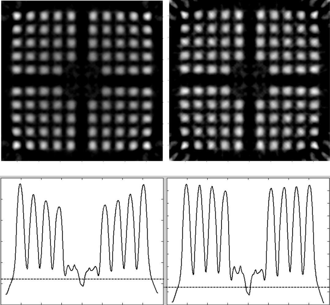
**Fig. 8:** Reconstructed images using simulated data. No correction was made for attenuation in the algorithm to the left while homogenous attenuation was incorporated into the algorithm developed in this work, yielding images to the right. Below are reconstructed pixel activities from the fifth row of fuel rods.
