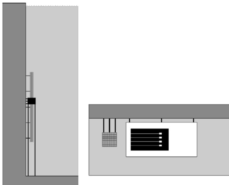
**Fig. 7:** A schematic layout of the proposed measurement geometry. The fuel assembly is rotated and lifted using an elevator system mounted on the wall of the fuel handling pool as shown in the left part of
