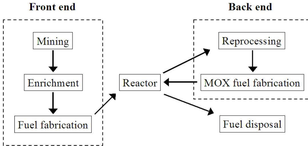
**Fig. 2:** Schematic illustration of the basic steps in the fuel cycle. The front end of the fuel cycle is represented to the left, i.e. mining, enrichment and fuel fabrication. The back end is represented to the right and involves the activities after reactor operation. The reprocessing, MOX fuel fabrication and further irradiation illustrates the closed fuel cycle.
