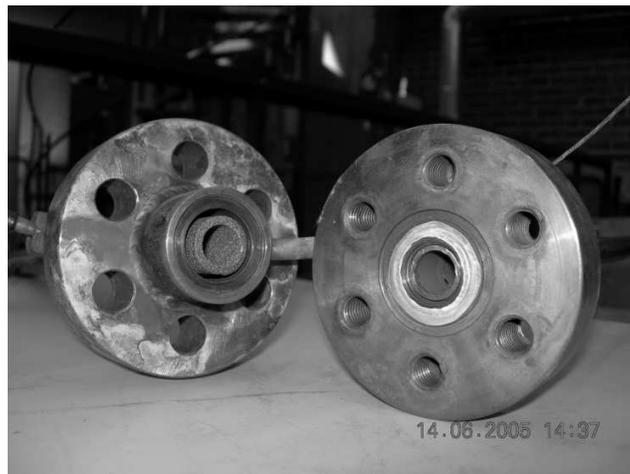
FIGURE 2.4. The porous sinter metal part mounted in the film extraction device.
