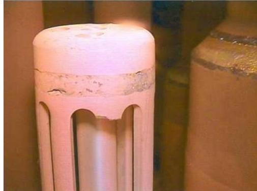
Figure 2: Corroded weld A182 at a protective cage – gable and lid are made of Alloy 600 and the visible part of the weld in Alloy 182 [14]
