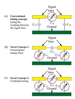
Fig. 1. Basic working principle of: (a) conventional tunable coupled line directional couplers, (b) novel Concept 1, and (c) novel Concept 2 of the MEMS tunable coupled line directional couplers presented in this paper.
