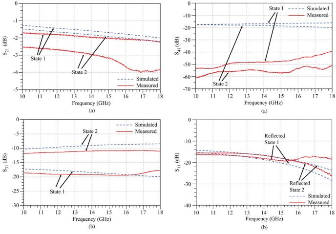
Fig. 14. Measured and simulated S-parameters in the two coupling states of 10–20-dB directional coupler (Concept 2). (a) Through  $(S_{21})$  port. (b) Coupled  $(S_{31})$  port.
