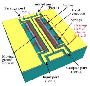
Fig. 2. Illustration of Concept 1, an ultra-wideband coupled line directional coupler based on geometrically tuning of the signal-to-ground coupling of the coupled lines.
