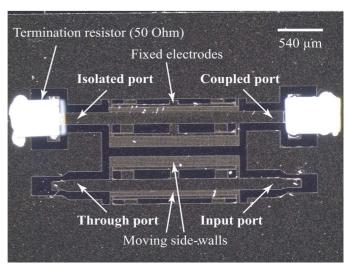
Fig. 10. Microscope photograph of a prototype device of Concept 2 in throughport measurement configuration, i.e., with the isolated and coupled port terminated by  $50-\Omega$  microwave-grade SMD resistors.
