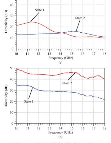
Fig. 17. Measured directivity for the fabricated directional couplers in the two coupling states. (a) 3–6-dB directional coupler (Concept 1). (b) 10–20-dB directional coupler (Concept 2).
