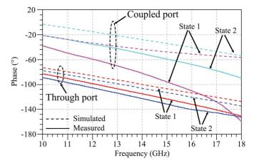
Fig. 16. Measured and simulated phase plots of coupled  $(S_{31})$  and through  $(S_{21})$  ports in the two coupling states of 10–20-dB directional coupler (Concept 2).
