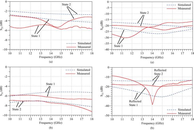
Fig. 11. Measured and simulated S-parameters in the two coupling states of 3–6-dB directional coupler (Concept 1). (a) Through  $(S_{21})$  port. (b) Coupled  $(S_{31})$  port.
