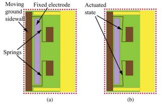
Fig. 3. Actuation states of Concept 1 (only one side of the coupled signal line illustrated). (a) State 1 (3-dB coupling). (b) State 2 (6-dB coupling).
