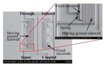
Fig. 8. SEM photographs of fabricated MEMS-tunable coupled line directional coupler of Concept 1, in 3–6-dB implementation, including a close-up view of the actuator.
