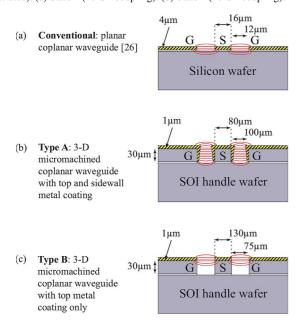
Fig. 6. Comparison of: (a) conventional 2-D coplanar waveguide, (b) 3-D micromachined coplanar waveguide of Type A with metallization layer on the sidewalls, and (c) 3-D micromachined coplanar waveguide of Type B with metallization only on the top layer.
