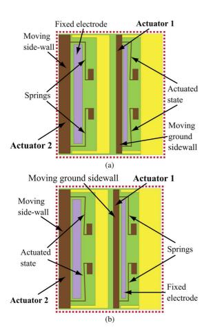
Fig. 5. Actuation states of Concept 2 (only one side of the coupled signal line illustrated). (a) State 1 (20-dB coupling). (b) State 2 (10-dB coupling).
