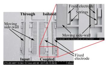
Fig. 9. SEM pictures of fabricated MEMS-tunable coupled line directional coupler of Concept 2, in 10–20-dB implementation, including a close-up view of the actuator.
