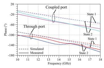
Fig. 13. Measured and simulated phase plots of coupled  $(S_{31})$  and through  $(S_{21})$  ports in the two coupling states of 3–6-dB directional coupler (Concept 1).
