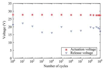
Fig. 19. Lifetime characterization: pull-in and pull-out voltages monitored over 1 billion cycles with 35-V unipolar square waveform with a 50% duty cycle and a cycle frequency of 1.6 kHz for measuring the pull-in/pull-out actuation hysteresis for each data point.
