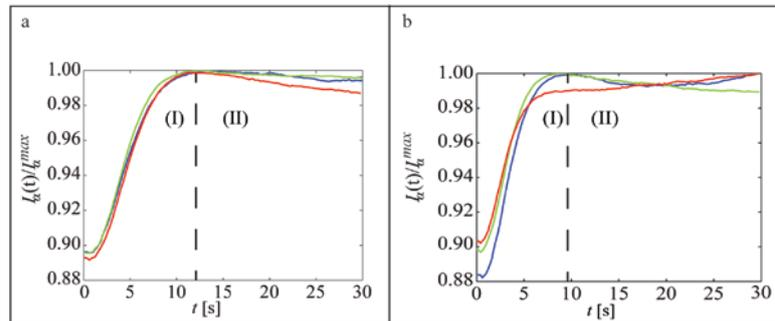
Figure 5: Reproducibility tests of the light intensity method. The diagrams are normalized light-intensity curves for a) single-frequency (SF) actuation, and b) frequency-modulation (FM) actuation. Each experiment was repeated three times.
