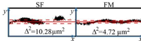
Figure 4: Analysis of the variance,  $\Delta^2$ , in final pattern shape. The dotted red lines mark the standard deviation ( $\pm\Delta$ ) of the pattern from an ideal straight line along  $x$  around its mean position ( $y_c$ ) (solid red lines). The variance is here defined as  $\Delta^2 = (1/N) \sum_{j=1}^N [y(x_j) - y_c]^2$ .
