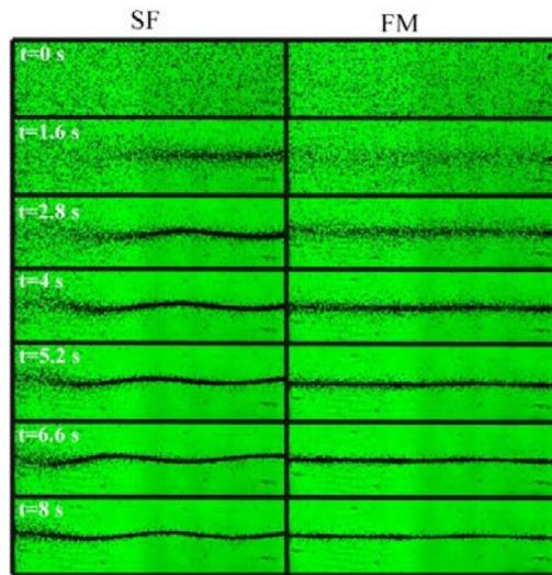
Figure 2: Dynamics of acoustophoresis patterns during the first 8 s when actuating the device with  $U_{pp}=20$  V at single frequency (SF, left panel) and frequency modulation (FM, right panel).
