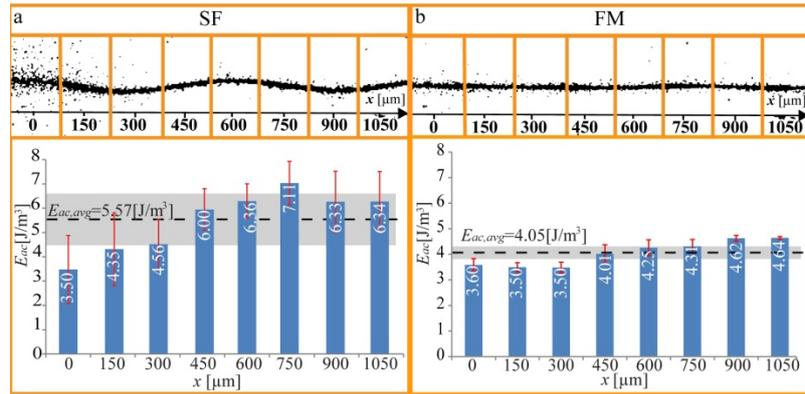
Figure 3: The spatial distribution in energy density along the channel for a) single frequency (SF) and b) frequency modulation (FM) actuation. The averaged energy density for the whole channel,  $E_{ac, avg}$ , is marked with a dotted black line, and the corresponding  $1\sigma$  standard deviation is marked with a grey band. The red error bars are the standard deviations from the four repetitions of each experiment.
