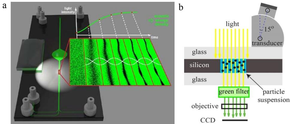
Figure 1: a) Illustration of the chip and the light intensity method for measuring the acoustic energy density. b) Schematic side-view of the device including the transducer with a 15° coupling wedge (not to scale).
