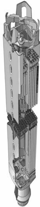
Figure 3.1: Illustration of a BWR fuel assembly with the fuel channel visible on the left side. Reproduced with courtesy of Westinghouse Electric Sweden AB.
